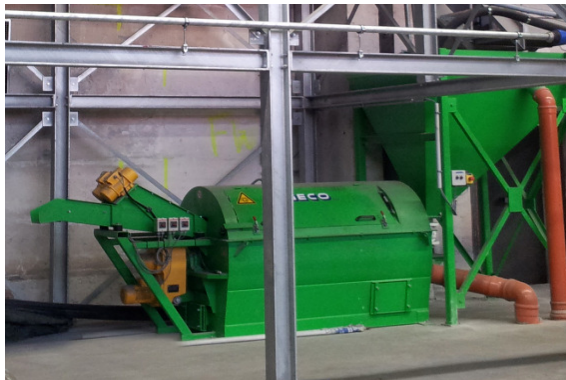
FLOTMAT-03-Vibro with preseparator and vibration chute.
