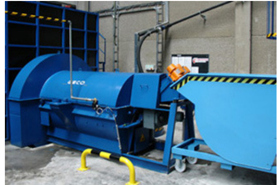
The drain chute conveys sand to a container with fixed wheels.
