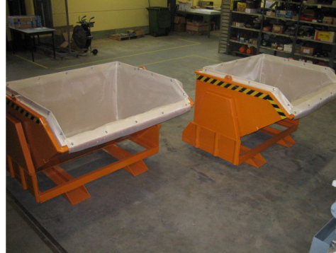
ECON-container to tilt facilitates the drawdown.
