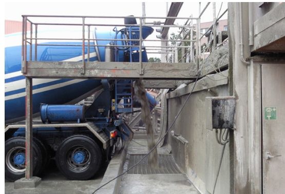
Infeed chute Cleaning device for 4 truck mixers at the same time.
