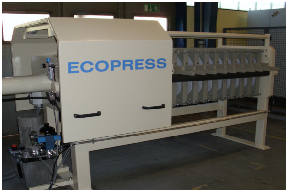
Fully automatic filtering by drip proof design and monitoring of the filling
