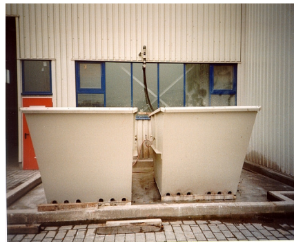
Efficient solution in a concrete stone plant. Alternate filling of two ECON containers allows an additional thickening of the sludge.
