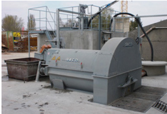
FLOTMAT-03-KOMBI with basin higher than the ground.
