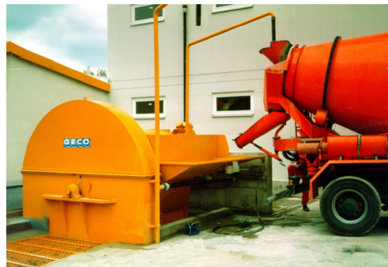
FLOTMAT-15-Kombi Feeding table for 2 truck mixers including cleaning device.
