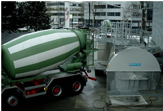
FLOTMAT-25-Kombi Feeding table at ground level to clean the court.
