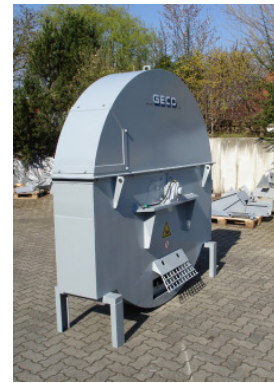
Feeding wheel as stand alone system.
