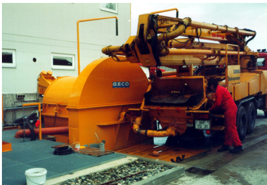
FLOTMAT-15-Kombi Feeding wheel for the cleaning of concrete pumps.
